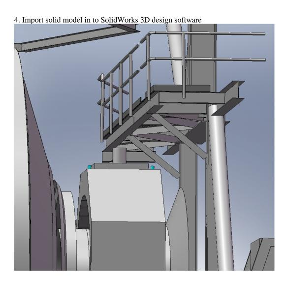
5. Design of platforms around scanned model in SolidWorks
